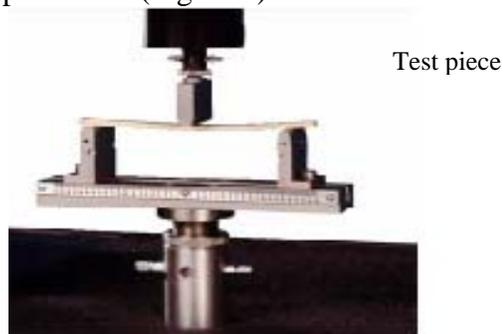
**Figure 1: Three-point bend test set up**
