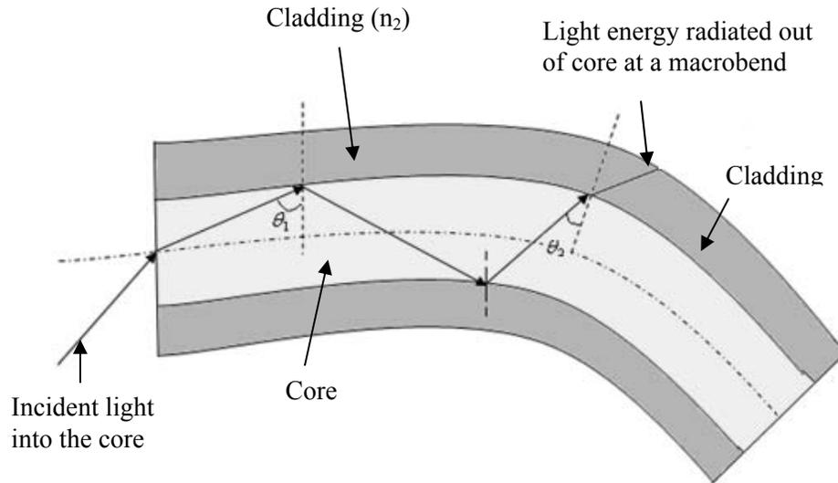
**Figure 1: Light Energy Radiated Out of Core at Macrobend
