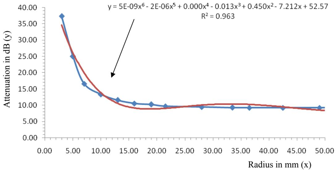
**Figure 4: Attenuation against Circular bend Radius**
