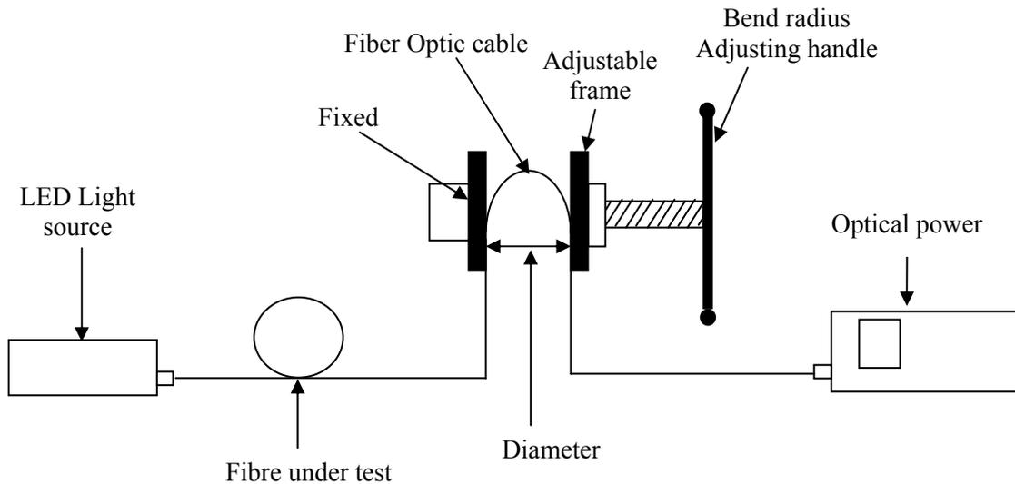
**Figure 3: Experimental Bending jig**
