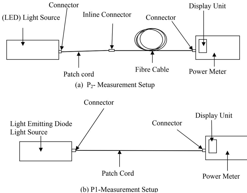
**Figure 2: Insertion Method Setup (Adapted from Bailey and Wright, 2003)**
