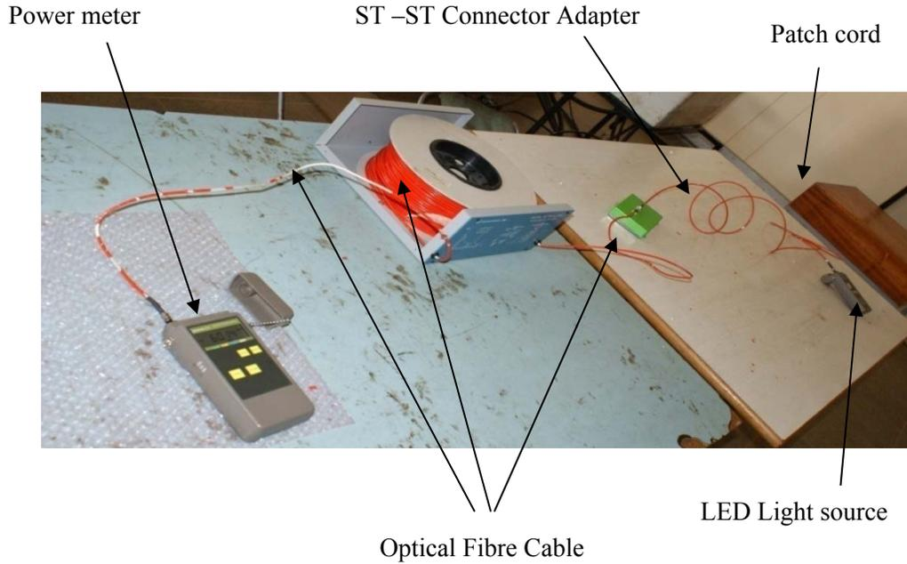
**Plate 3.1** Experimental Setup for  $P_2$  Measurement
